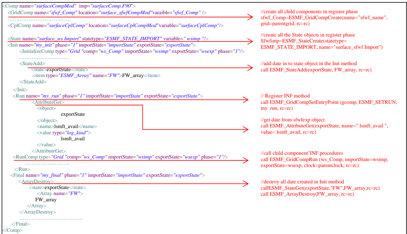
Figure 7. Mapping between ESMCDL and code for forcing Gridded Component
