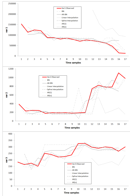
Fig. 4. Example of the missing data estimation using the different techniques. The example corresponds to the 3 different variables of Dataset 2 respectively for an RMD scenario. For this example, each sample of the time series is hidden one at a time, and the missing sample is estimated using the rest of the series as necessary by the different estimation techniques.
