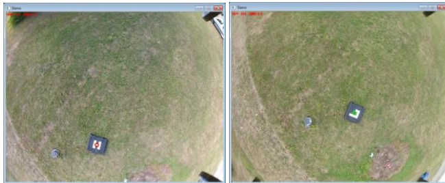
Figure 4. In-flight detection of shape "H" and "L" marked by colored circles at the center of the pattern ("H" is marked red; "L" is marked green)
