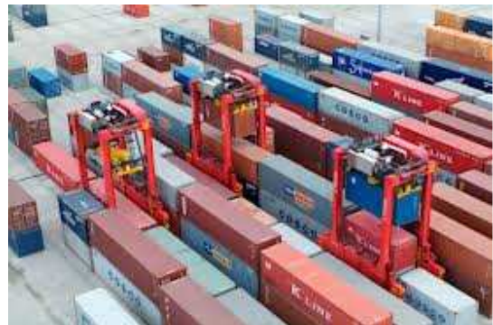
Fig. 1 Straddle carriers circulating in a containers yard
