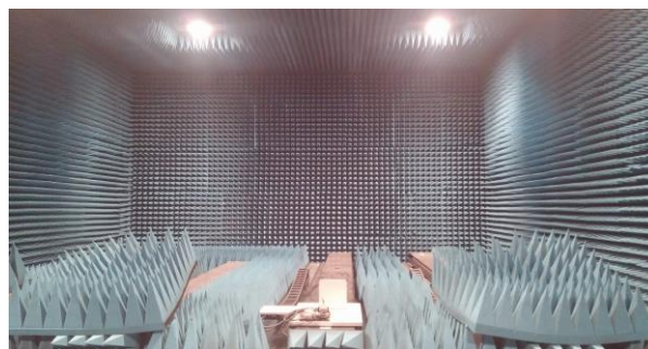
Figure 8. Used anechoic chamber for the performance measurement
