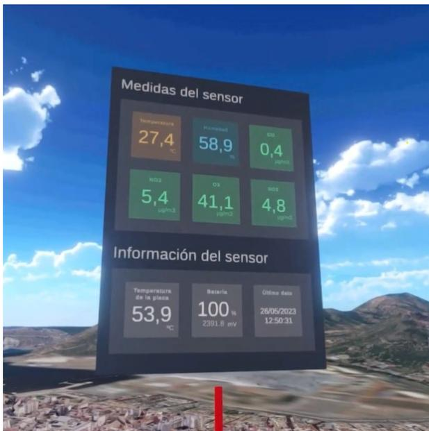
Figure 9. Unity object displaying air quality data from sensor devices.
