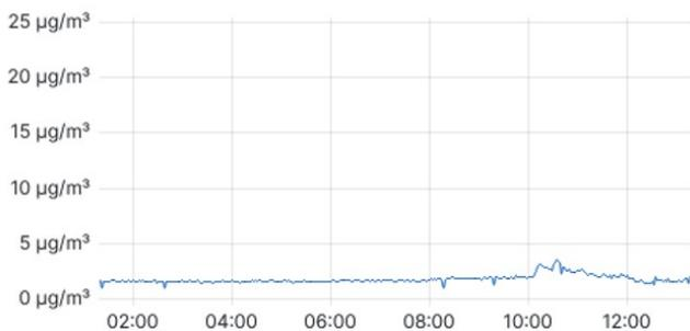
Figure 2.  $PM_1$  data from suspended particulate matter device.
