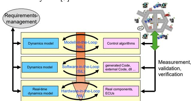
Figure 1. Seamless model-based development and validation process[6]
