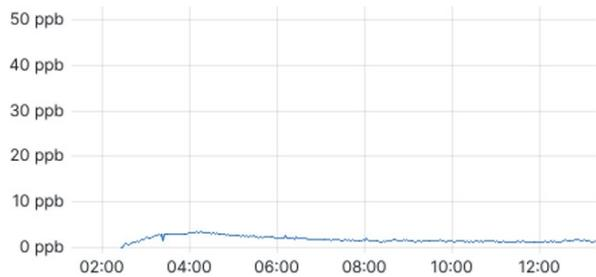
Figure 8. NO<sub>2</sub> data from pollutant gas monitoring device.
