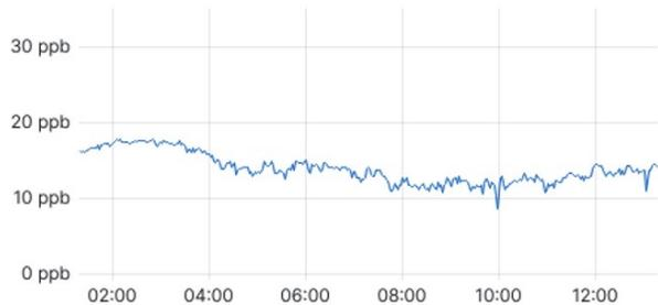
Figure 6. SO<sub>2</sub> data from pollutant gas monitoring device.
