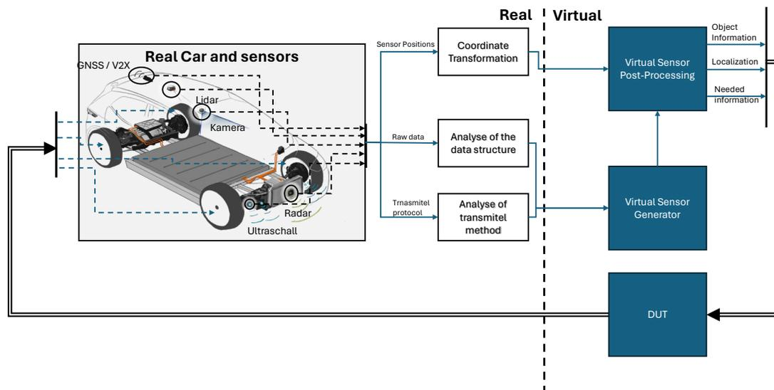
Figure 2. Concept of the sensor simulation and post-processing
