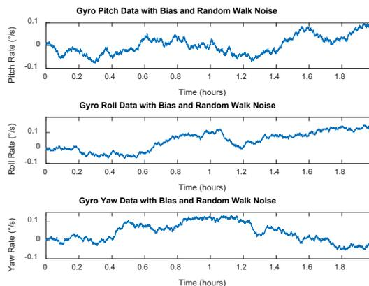
Figure 7. Noisy IMU data - angular velocity
