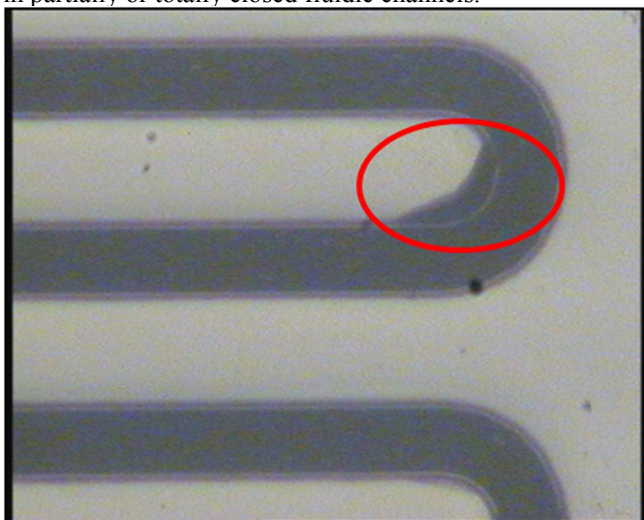
Figure 7. Effects of insufficient exposure time. The circle points an obvious underexposure effect on the TMMF structure.
