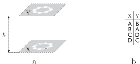
Figure 6. The noncoplanar layout of tQCA cells (a) and the result of cell to cell interaction (b).
