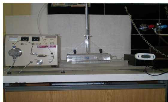
Figure 4. Analytical miniaturised system with micropump(left), separation microcolumn (middle) and fluidic channel with nanostructure in deposition cell (middle bottom).
