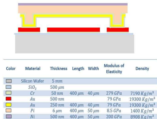
Figure 3. Cross sectional view of the fabricated microbeam.
