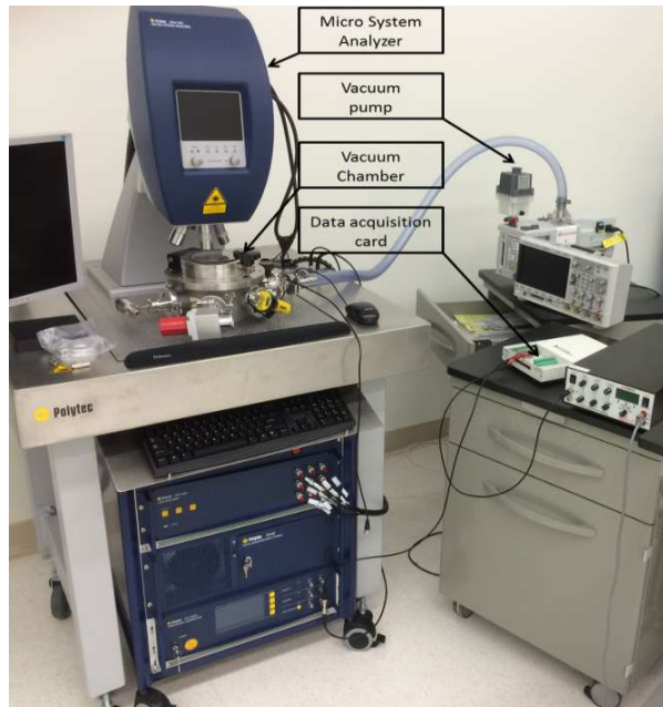
Figure 4. Experimental setup used for testing the MEMS device.
