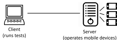
Figure 1. Client-server interaction in a mobile testing environment.
