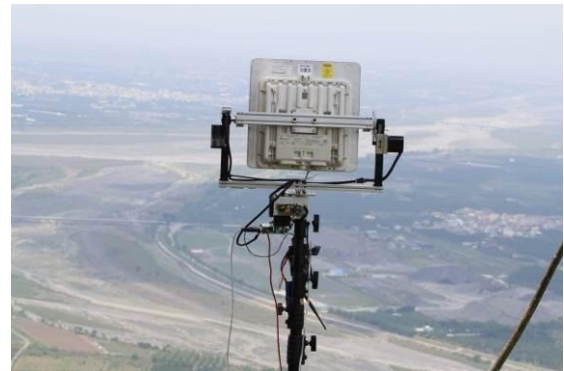
Figure 11. Ground terminal tracking unit with microwave module.
