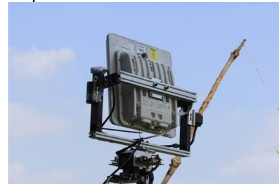
Figure 5. Two-axis Stepper Motor Rotation Platform.
