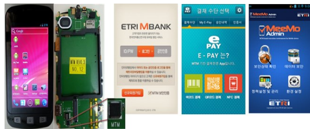
Figure 3. MTM based mobile device and secure service applications
