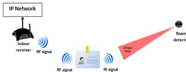
Figure 4. Overview of the indoor positioning system
