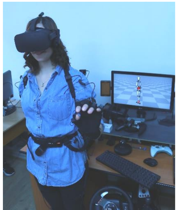
Figure 4. Experimental setup and sensor fusion results. Test-person in front of VR station wearing Oculus Rift headset with Neuron Perception suit.
