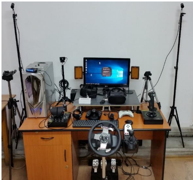
Figure 1. Virtual Reality station and reference sensors. The steering wheel and throttle and stick levers are not used in this particular set of experiments but they are employed for other behavioral studies using virtual reality in biomedical applications.
