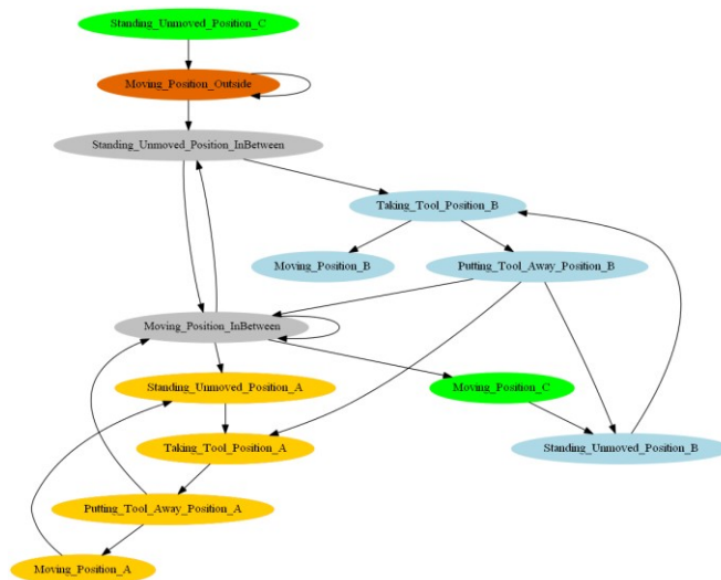
Figure 9. Identified process model of the second sequence of the second scenario. Different colors represent different places: Yellow – A, Blue – B, Green – C, Grey – In Between, and Red – Outside.
