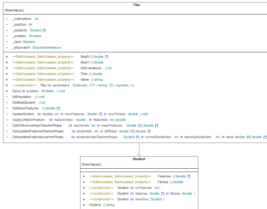
Figure 2. The implementation of the Teaching-Learning based Optimization algorithm (UML class diagram).
