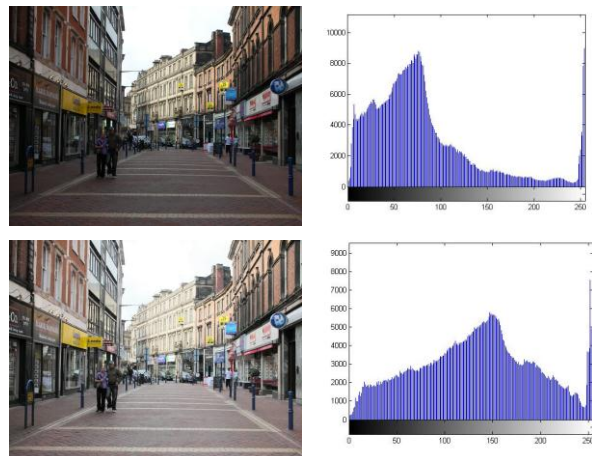
Figure 3. First row: original image and its luminance histogram; second row: processed result from our global contrast enhancement method and its luminance histogram.
