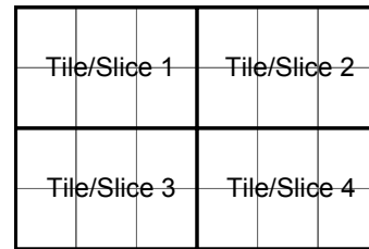
Figure 5. The picture is divided into 24 CTUs and into 4 Slices as well as 4 Tiles of equal size. Each Tile and each Slice contains 6 CTUs.
