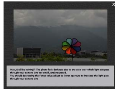
Figure 12. An example of bad settings (too dark) of aperture F/22 and shutter speed 1/1000.
