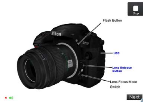
Figure 3. Several components of 3D DSLR camera are labeled with hotspots.
