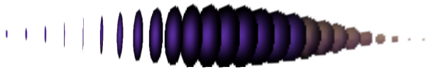
Figure 2: A video grain, the windowing function is applied on the spatial and temporal dimensions.
