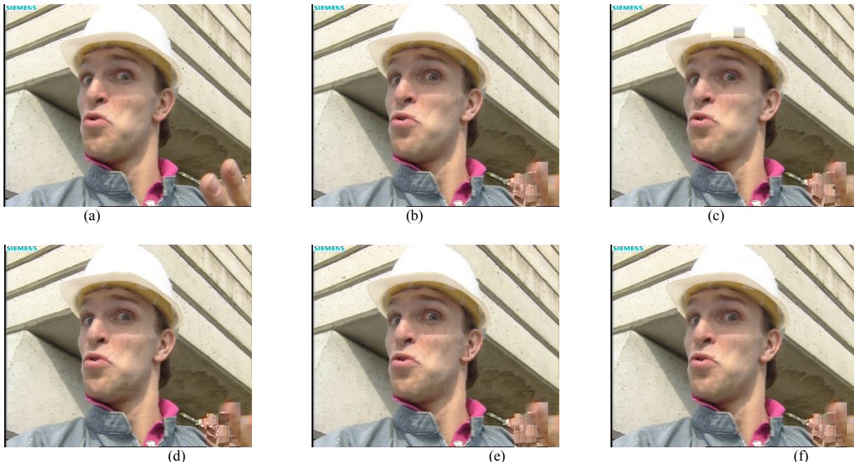
Figure 2. Sample results for the “foreman” sequence when the motion block size is 16 \times 16 and the search range is \pm 16 . (a) Original frame, (b) Reconstructed frame with the SAD based ME (PSNR = 30.48dB) (c) Reconstructed frame with the MCW2BT-LS ME (PSNR = 29.56dB), (d) Reconstructed frame with TGCBPM with NTB = 5 (PSNR = 29.91dB), (e) Reconstructed frame with WTGCBPM with NTB = 5 (PSNR = 29.72dB), and (f) Reconstructed frame with the proposed MCGCBPM-LS with NTB = 5 (PSNR = 30.36dB)
