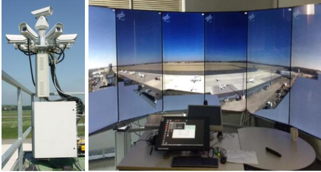
Figure 1. DLR Remote Tower field test platform at Braunschweig-Wolfsburg Airport (BWE) (left: Camera sensors; right: ATCO working position).
