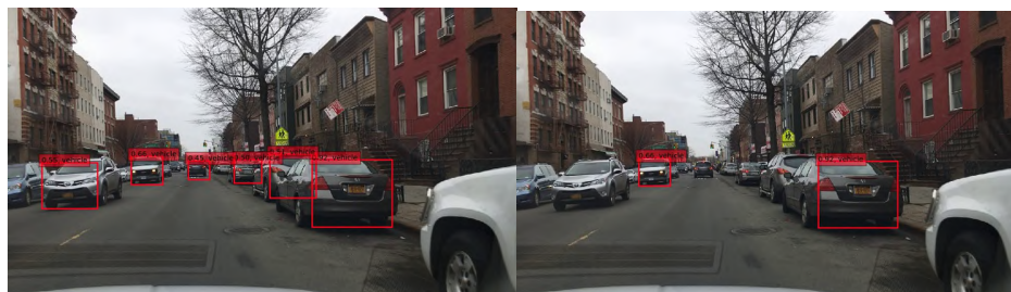
Figure 2. Detected concepts by the network with a low threshold (0.4) on the left and a high threshold (0.6) on the right.
