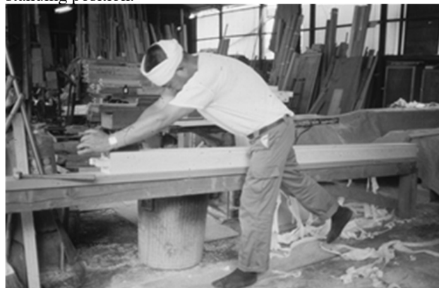
Figure 2. Half body (diagonally opposite to the planing material).
