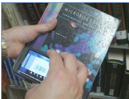
Figure 6: AoE Library Navigator: Tag Based Information Search: Scanning the book barcode initiates a web based search
