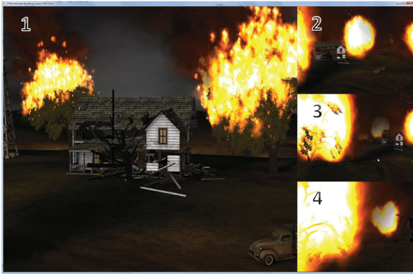
Fig. 2. The result of multi-view rendering with different resolutions (1: 1600x1440, 2,3,4: 640x480)
