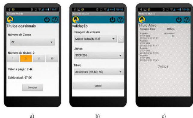
Figure 2. Mobile payment system screens: (a) buy ticket by choosing the type (zone); (b) validate ticket; (c) active ticket (interfaces in Portuguese).
