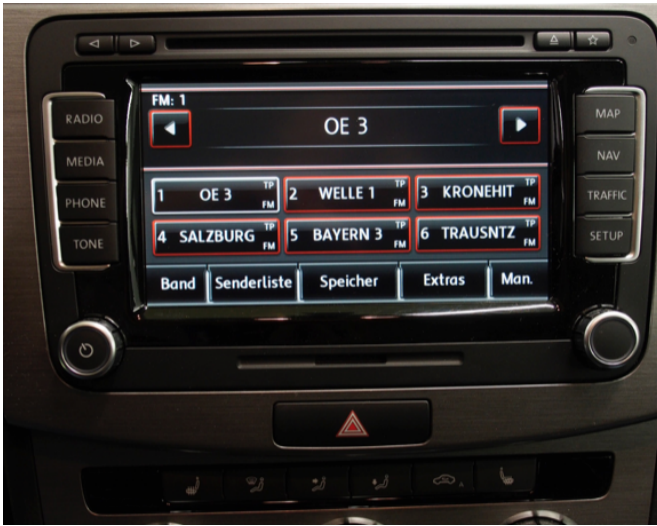
Figure 9. VW Passat dashboard which combines few physical buttons with a well-readable touch display.
