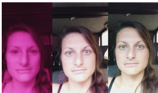
Figure 4. Indoor (bright light) - NIR only, NIR & visible light, visible light only (from left to right).
