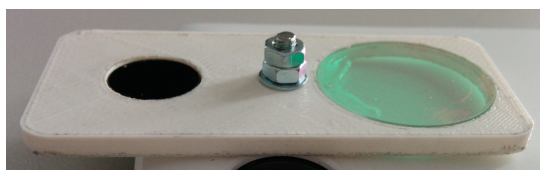
Figure 8. Final lens holder mounted on the phone case.
