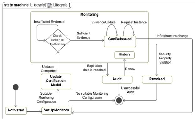
Figure 2: Life cycle of incremental certificates
