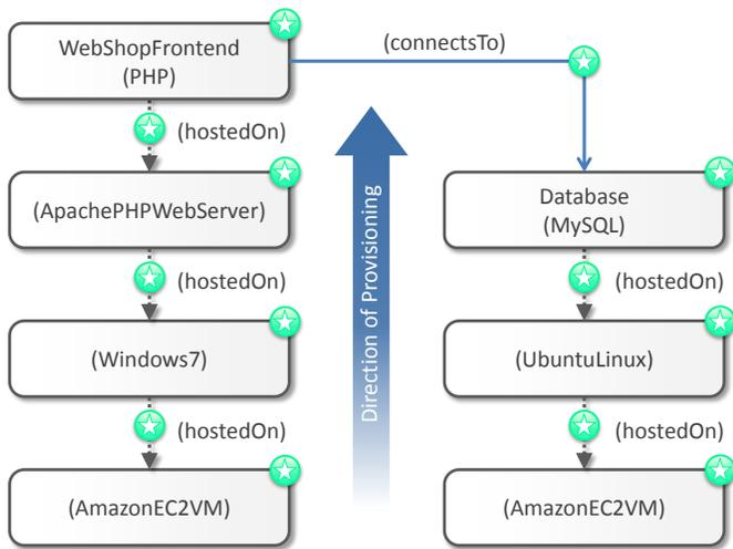
Figure 3. Annotated application topology to be provisioned.
