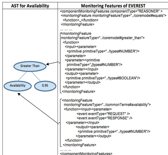
Figure 6: Availability AST and matching monitoring configuration
