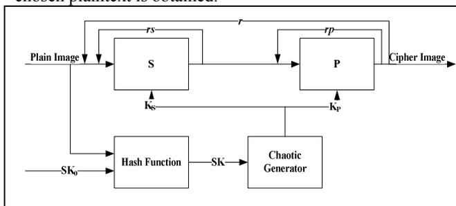
Figure 1. Encryption Parts of the Proposed Cryptosystem
