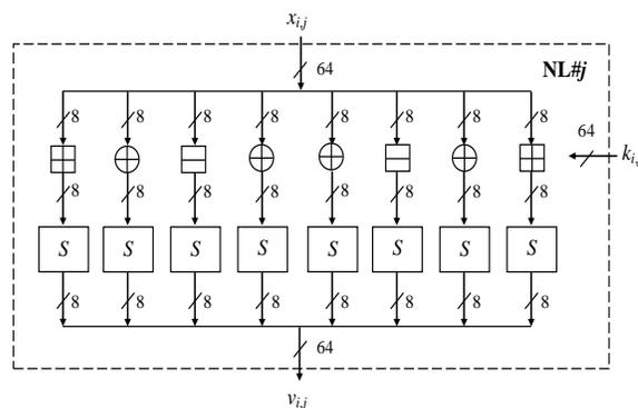
Figure 2. Nonlinear element  $NL\#j$  of PP-2 ( $j = 1, 2, \dots, t$ )
