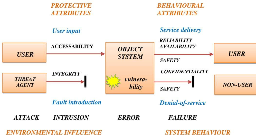
Fig. 1. An integrated model of security and dependability
