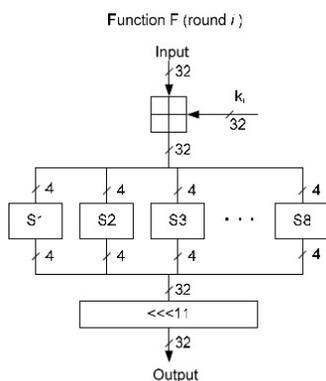
Fig. 2. Detailed description of the round function  $F_i$  used in GOST
