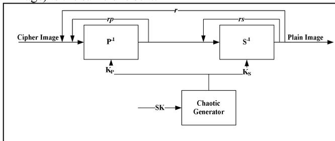
Figure 2. Decryption Parts of the Proposed Cryptosystem
