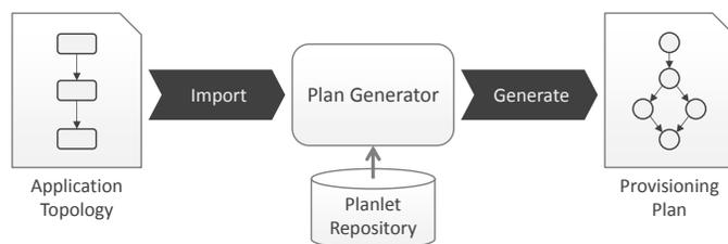
Figure 2. Management Framework for generating Provisioning Plans.
