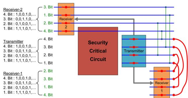
Figure 2. Illustration of bypassing the regular active shield.
