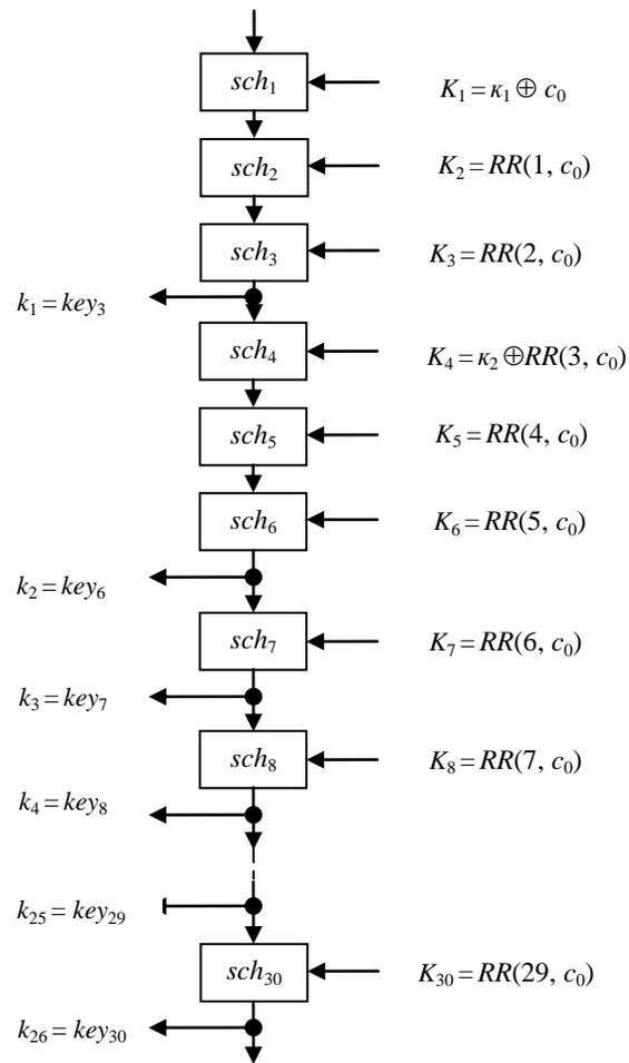
Figure 7. The scheme of the generation of round keys for  $n = 128$  and  $|k| = 256$
