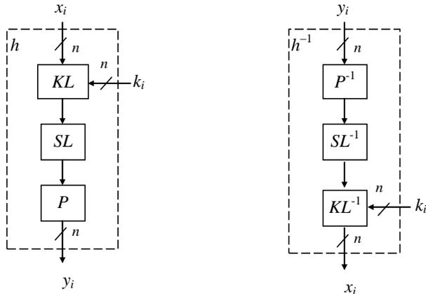
Figure 3. Round function  $h$  (encryption) and its inverse function  $h^{-1}$  (decryption)
