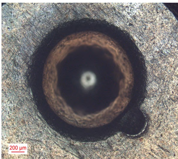
Figure 8. Image of mark after firing pin on cartridge case fired from Walther PPQ measured with optical microscope.
