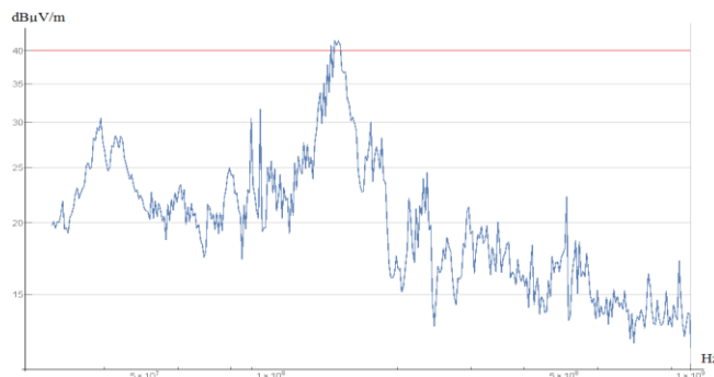
Figure 6. GTEM cell - the EMI of the EUT in the state of alarm
