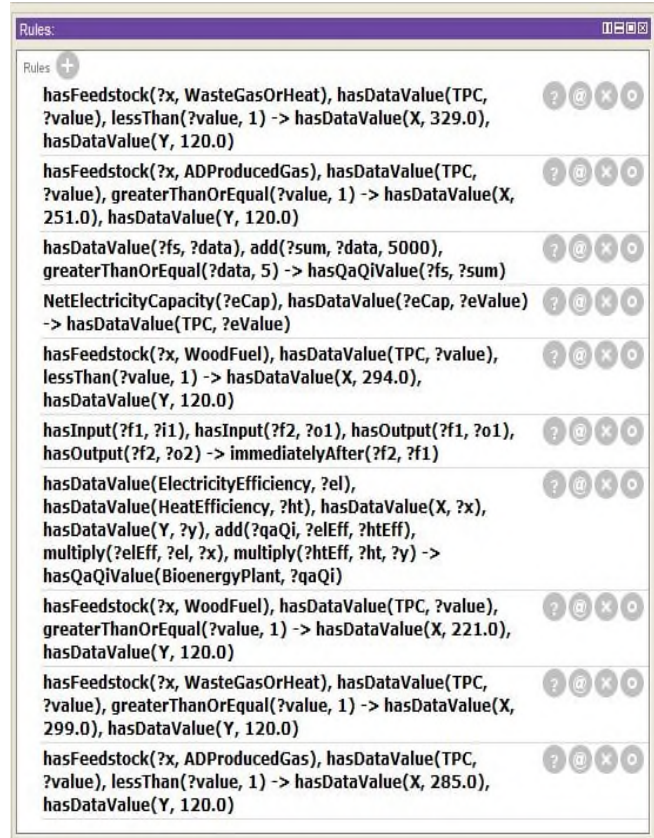
Figure 4. Some SWRL rules in Protégé to assert new knowledge and calculate the quality assurance
