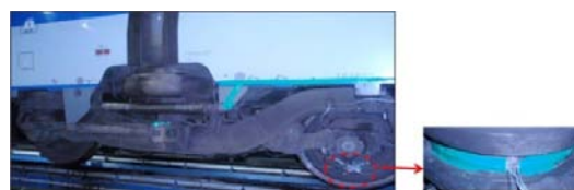
Figure 1. The temperature measuring on the axle box bearing
