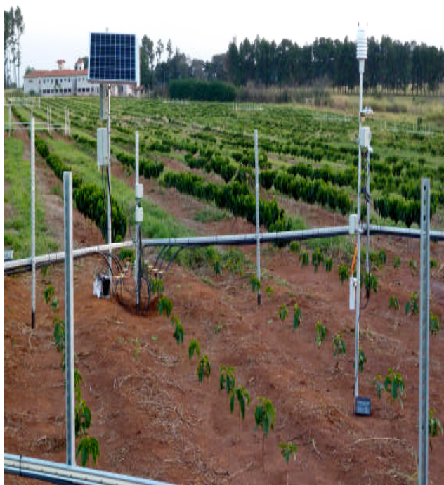
Figure 4. Partial view of one FACE plot showing the adapted devices: 1) one CO 2 probe and one weather station at the plot center and 2) one flow controller and eight valves, one for each octagon section, positioned at the south border. The general-purpose circuit is inside the small plastic boxes. A 65 Watts photovoltaic panel has been used to supply power for each plot.
