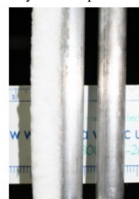
(b) Ice formation at the windward side of the cylindrical probes
