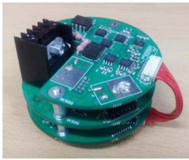
Fig. 3. Implemented acoustic transceiver.
