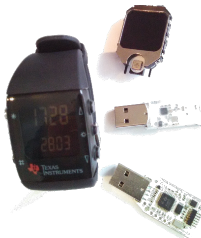
Figure 1. Texas Instruments eZ430 Chronos - Development Kit
