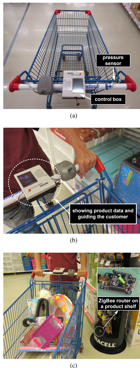
Figure 5. IST system deployment in Carrefour: (a) encapsulate all components into a control box, (b) the LCD touch panel shows the product data and guide the customer (by the moving direction), and (c) the shopping trolley communicates with the ZigBee router placed in a product shelf.
