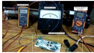
Figure 12. Measurement set-up for constant DC current source
