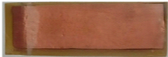
Figure 1. PMMA coated CPI sensor on polyimide PCB substrate.
