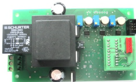
Figure 10. The PCB with all controlling and measuring electronics of a three sections sensor.
