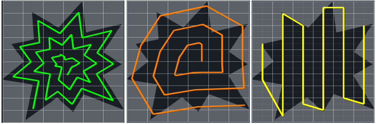
(a) Trajectory by Basic Spiral motion (b) Trajectory by Spiral convex hull (c) Trajectory by our work
