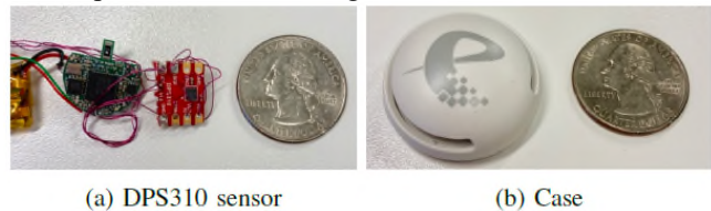
Figure 2. The proposed fall detection sensor node, which consists of a BSN node, a battery, and a casing of the sensor (with a quarter US dollar coin on the side)
