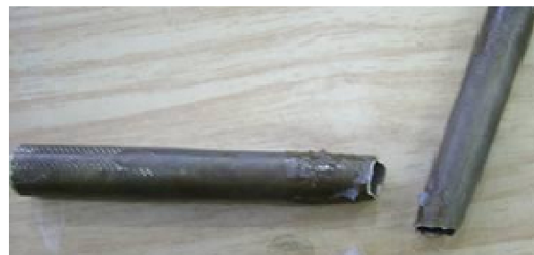
Figure 9. Brass pipe after stretch cracking ( \phi 10x150 mm and 0.5 mm thickness).
