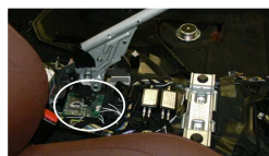
Figure 8. Sensor module on HIFI control unit (picture courtesy of BMW Group München)
