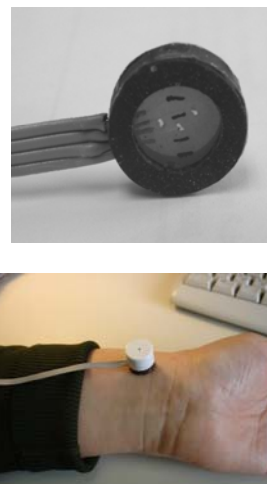
Figure 3. Photo images of the blood-pulse sensor (Top) and sensor location on the carpus of a volunteer under pulse testing (Bottom).
