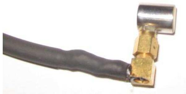
Figure 4. AE piezoelectric sensor.
