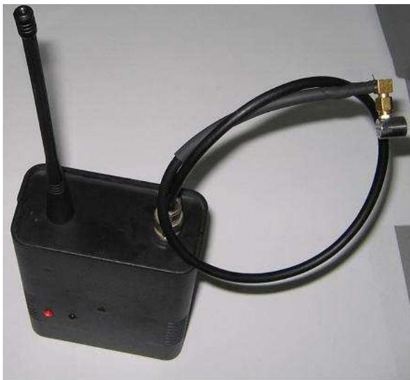
Figure 5. Experimental wireless module for acoustic emission sensor.
