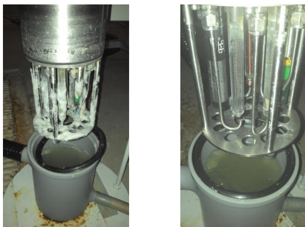
Figure 3. Multi sensor system to control process water of the paper industry left contaminated; right after cleaning with compressed air
