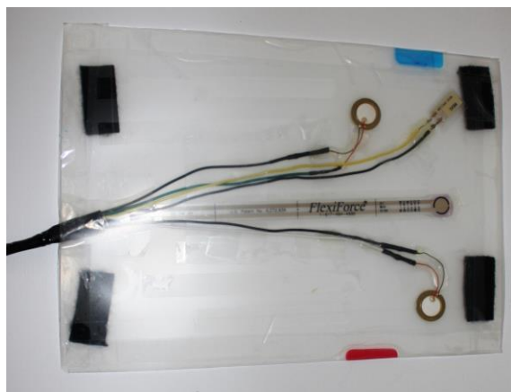
Figure 1. Sensor pad. (a) Vibration sensor; (b) Pressure sensor; (c) Velcro that is used to help the sensor pad stay in position.
