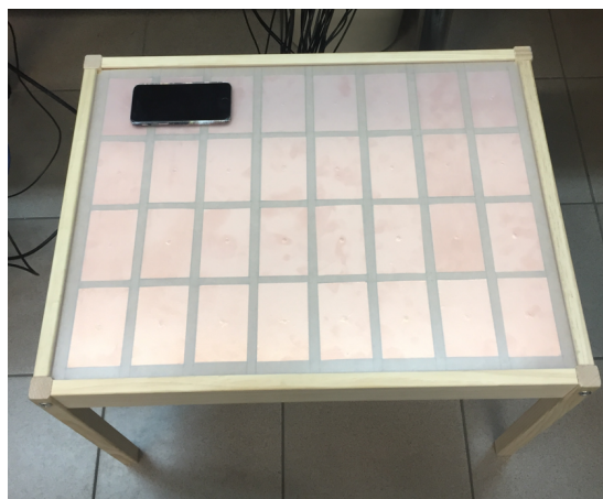
Fig. 1. Photo of TomoSense - top view of the system with a single mobile device (iPhone 6) placed on the table. Note the size of the sensed surface relative to the smartdevice.
