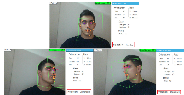
Figure 5. The GUI displaying the classification considering different poses (results using Gaussian SVM method). The classifier output is presented in the interface (red rectangles).
