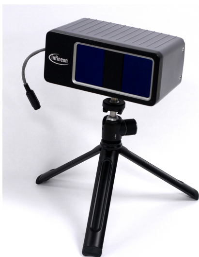
Figure 9. 1D MEMS mirror based LiDAR prototype.
