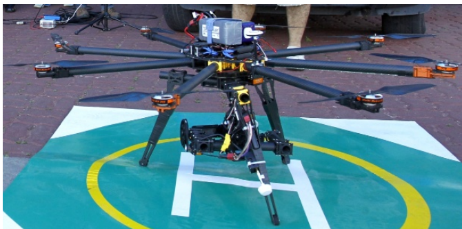
Figure 2. The multirotor has a camera with an infrared viewfinder attached for night monitoring, and a transmission link to enable real-time monitoring of images.
