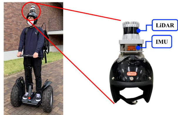
Figure 1. Overview of the experimental smart helmet.
