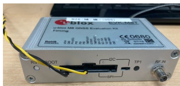
Figure 13. GPS module overview.
