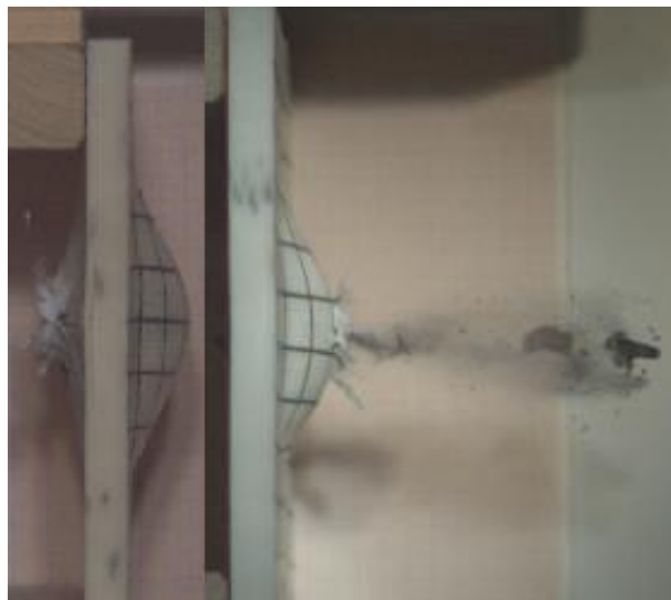
Figure 6. Effect of 60 plies Dyneema®HB26 impacts by a 7.62×39 mm FMJ bullets at 20 °C (left) and 110°C (right), 265 μs and 53 μs after the initial impact.
