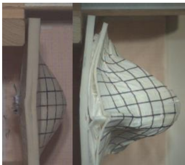
Figure 7. Effect of 60 plies Dyneema®HB26 impacts by a 7.62×51 mm FMJ bullets at 20 °C (left) and 110°C (right), 409 μs and 2050 μs after the initial impact.
