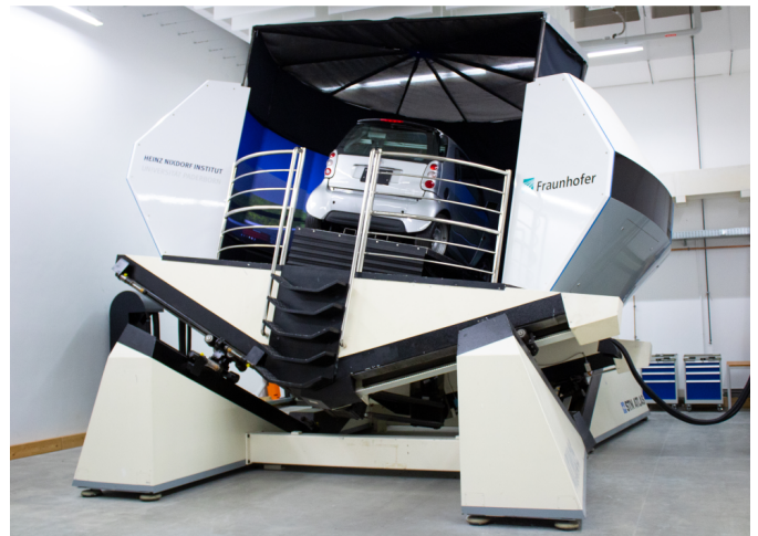
Figure 2. ATMOS Dynamic Driving Simulator.
