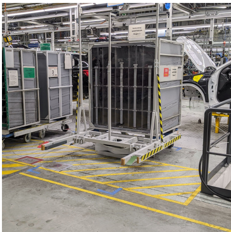
Fig. 3. Exemplary two-bin principle: the full container is facing the production line. The empty container has already been collected. Replenishment will be delivered shortly.
