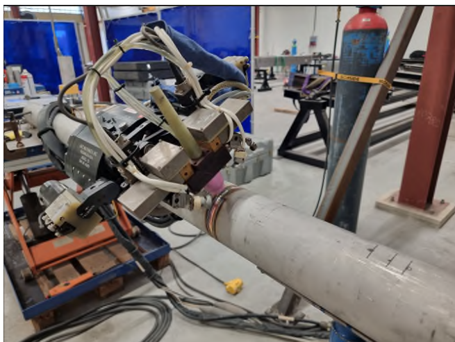
Figure 1. Orbital TIG Welding head mounted on a pipe during experiments.
