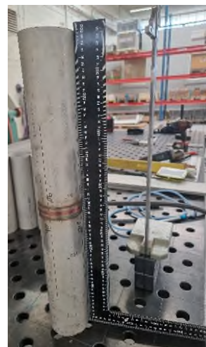
Figure 11. Straightness in pipe after welding.
