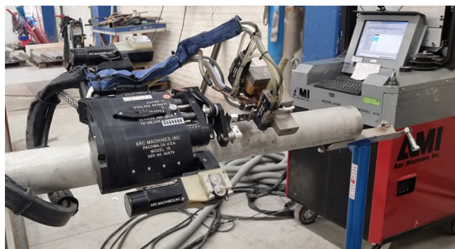
Figure 4. Welding head, Arc Machines Inc. Mod. 15.
