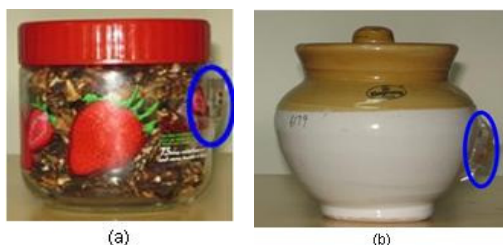
Figure 8. Tag attached with air gap in (a) Glass container and (b) Porcelain container.
