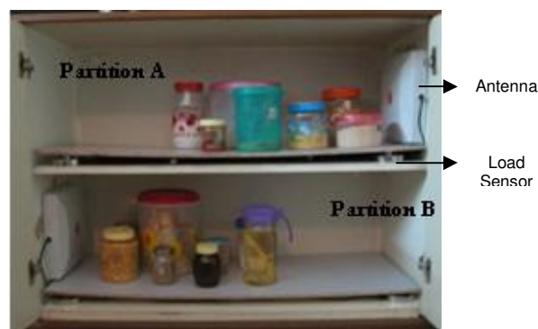
Figure 2. Deployment of Smart Kitchen Cabinet in C-DAC, Guest House.
