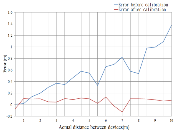
Figure 6. Calibration of localization error
