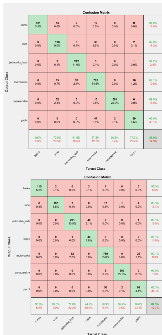
Figure 2. Exemplary confusion matrices for different number of classes in pre-trained GoogleNet solution [4]
