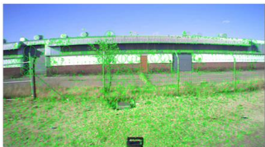
Figure 6. Detecting the image feature using SIFT.
