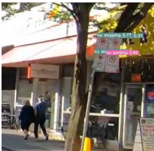
Figure 5. An example of YOLOv7X's ability to accurately detect several signs even at very poor visual quality.
