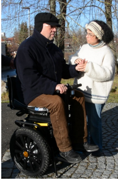
Figure 2. The photo shows the test driver on the vehicle, receiving a short briefing on how to steer the AddSeat® sighted guide using Lorm fingerspelling.
