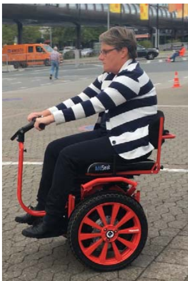
Figure 2. The photo depicts one of our blind test persons outdoors in a full stop emergency brake action.
