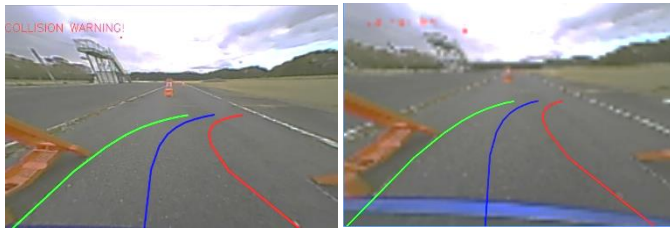
Figure 11. Camera images (Left: 1001 \times 667 , Right: 100 \times 67 )
