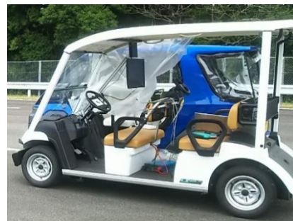
Figure 9. The vehicle with remote type automated system
