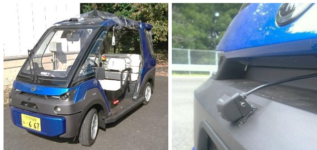
Figure 8. Automated vehicle (Left: Electronic vehicle, Right: Front camera)
